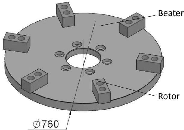
**Figure 2** Working components – beaters and rotor
