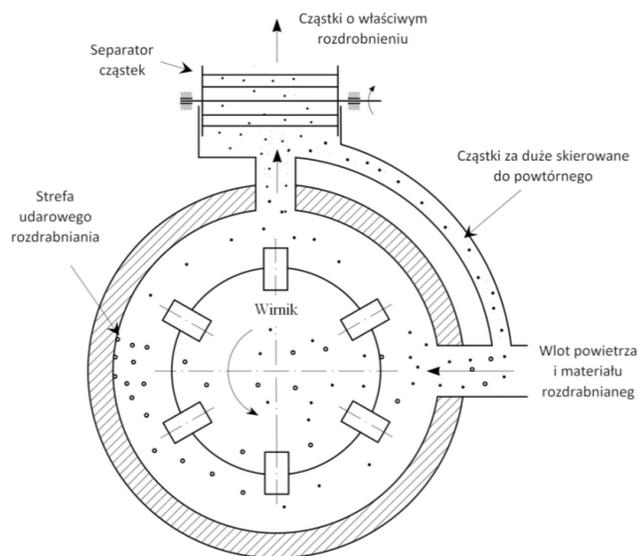
**Figure 1** Operational diagram of a rotor mill with particle separation
