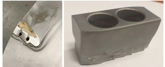
**Figure 4** View of the rotor mill's working components after 60 hours of operation (micronised material – oat seed coats, humidity <8%)
