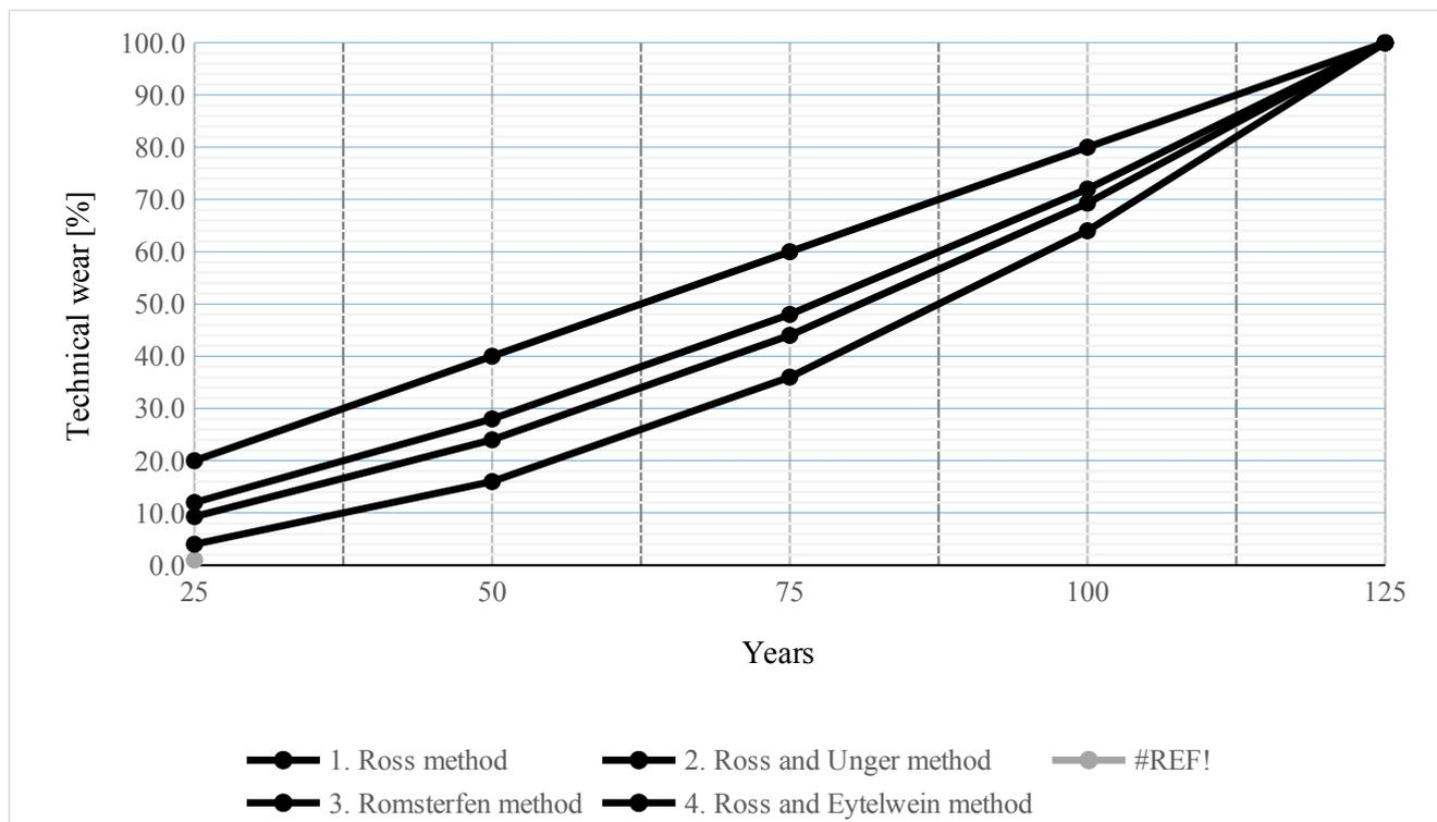
**Figure 3** Percentage of technical wear of a precast large-panel building according to the quality of operations and maintenance
