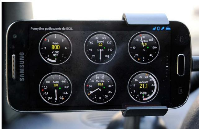
Figure 7 Smartphone Samsung Galaxy 4 Mini running Torque Pro
