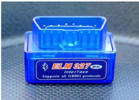
Figure 6 Bluetooth Wireless Diagnostic Interface ELM-327
