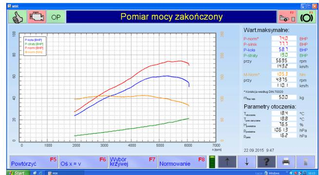
Figure 8 Results of power measurements on chassis dynamometer
