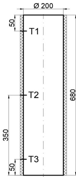
**Figure 3** Layout of the temperature sensors: T1, T2, T3
