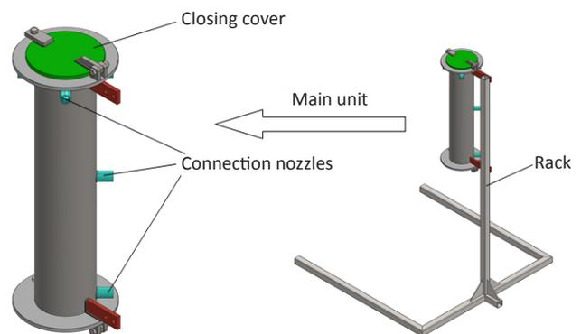
**Figure 1** Diagram of the stand for testing the sterilization process of food raw materials
