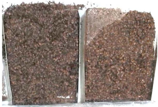
**Figure 4** Heat treated cocoa shell (heat treatment time: 2 min). Left side: 300°C, right side: 200°C
