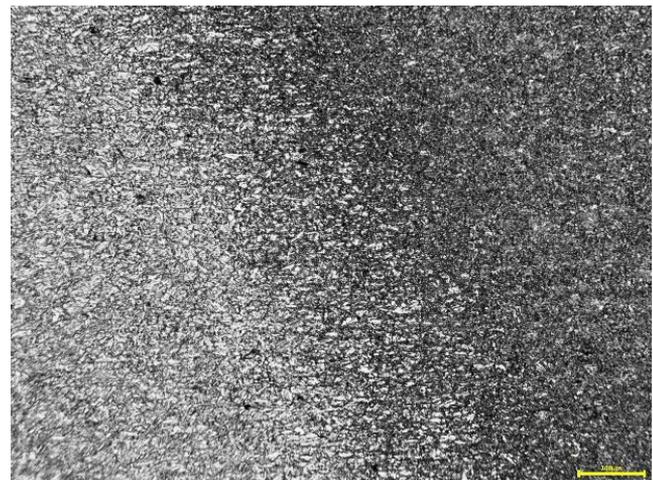
**Figure 1** Structure of the weld made using Union X90 welding electrode and a shielding gas mixture Ar + 10% CO<sub>2</sub>
