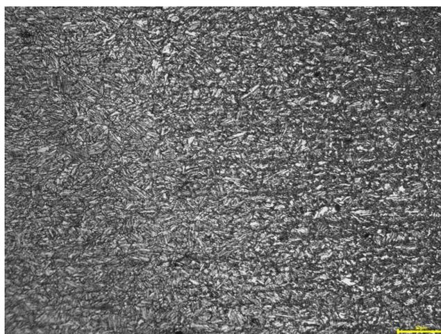
**Figure 1** Microstructure of a MIG welded DOCOL 1200M steel weld made using Ar as the shielding gas at preheating temperature of 80°C and welding velocity of 400 mm/min
