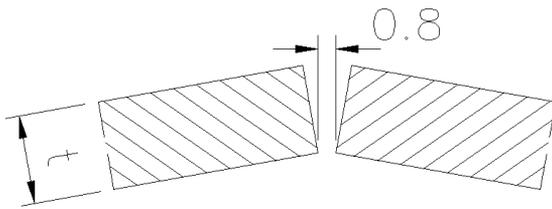
**Figure 1** Method of preparation of the joint for MAG welding
