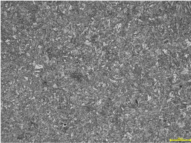
**Figure 2** Microstructure of a MAG welded DOCOL 1400M steel weld made using shielding gas (82% Ar + 18% CO<sub>2</sub>) at preheating temperature of 80°C and welding velocity of 300 mm/min
