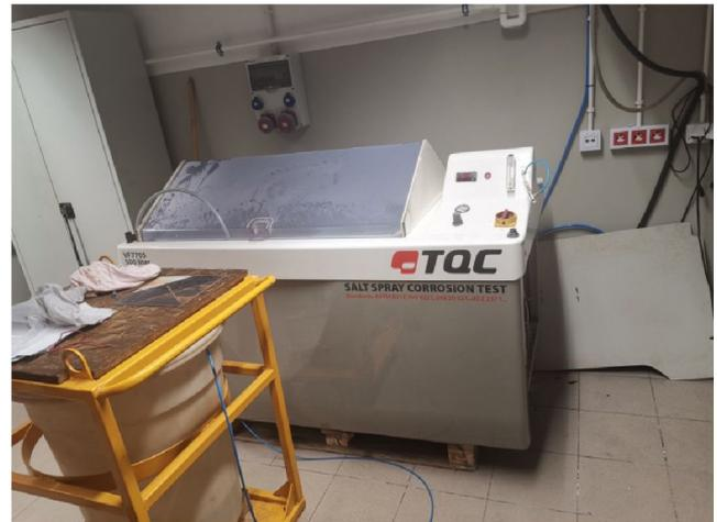
**Figure 1** Photograph of the salt spray chamber in SaMASZ.
