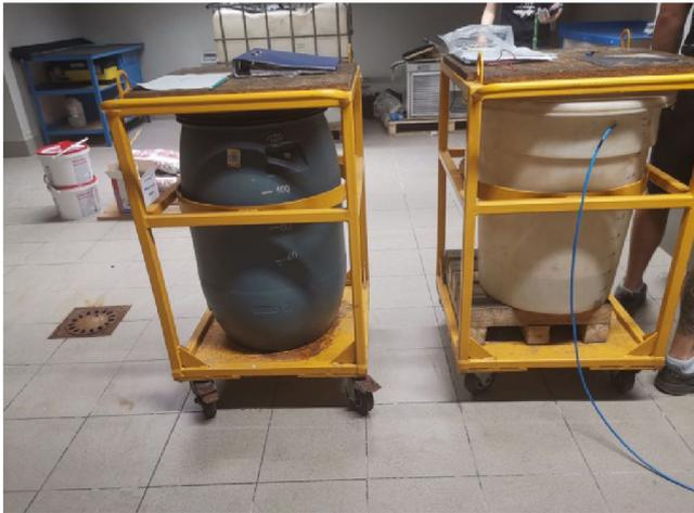
**Figure 2** Salt spray tank.
