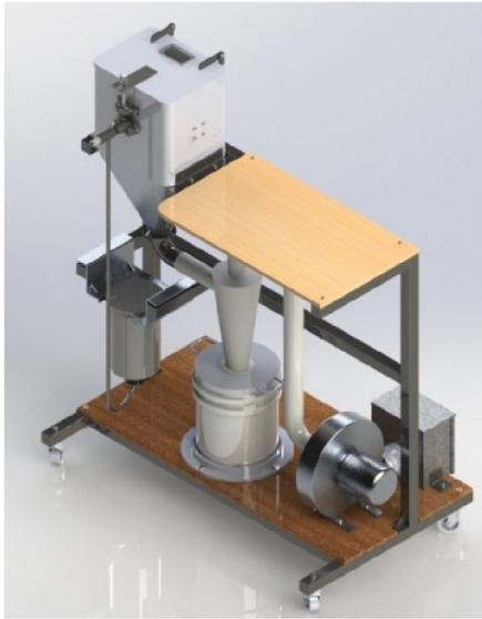
**Figure 3** Visualisation of the design of the didactic stand for testing the erosion process developed in SolidWorks
