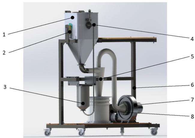
**Figure 1** Diagram of mobile didactic stand for testing the erosion process
