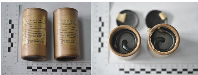
**Figure 2** Original military fire-cracker with fuse detonator (authors photo)
