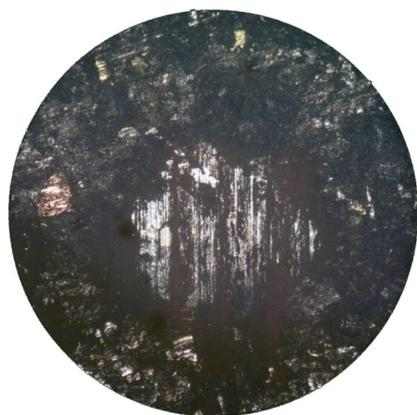
**Figure 6** A microscope photo of one of the craters formed during the tests
