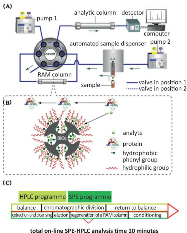
**Figure 4** A scheme of an automated SPE-HPLC system (A), the principle of extraction and cleansing of a RAM column (B), the idea of the whole SPE-HPLC procedure (C) [15]
