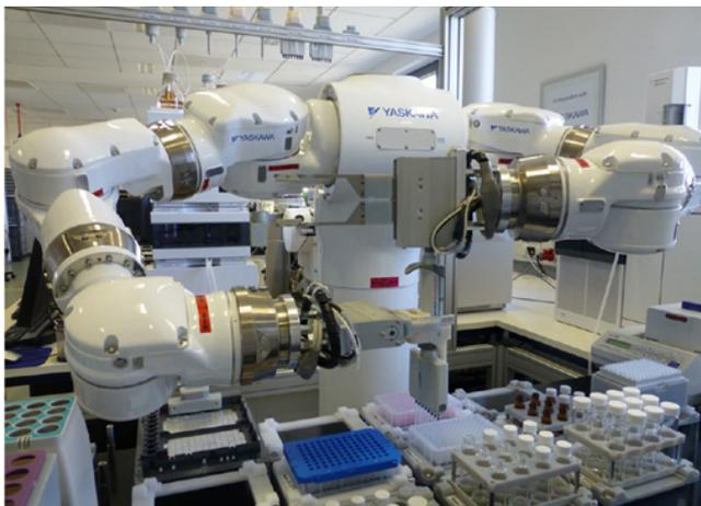
**Figure 6** A dual-arm SDA10F robot pipetting with a manual multi-channel pipette [20]
