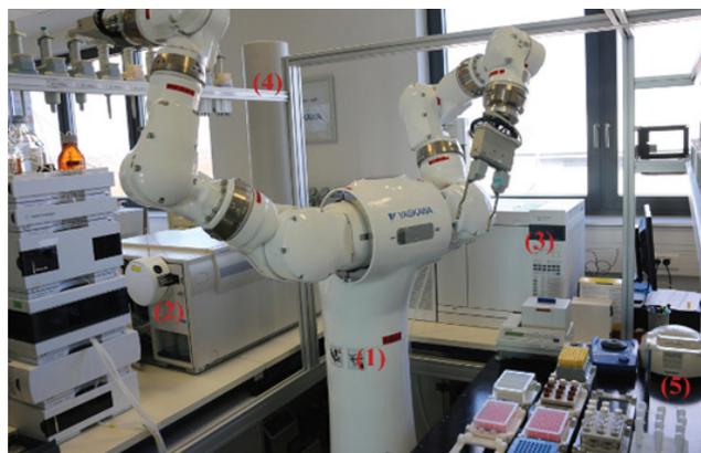
**Figure 5** A dual-arm CSDA10F robot (1) lifting a pipette, (2) LC/MS, (3) GC/MS, (4) a shelf with pipettes, (5) a sample preparation stand before transferring them to an analyser [19]
