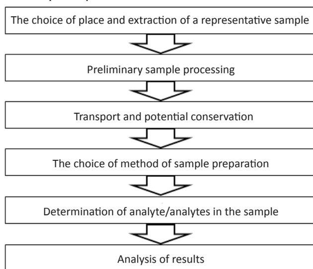
**Figure 1** A scheme of a procedure of determining analytes [1]
