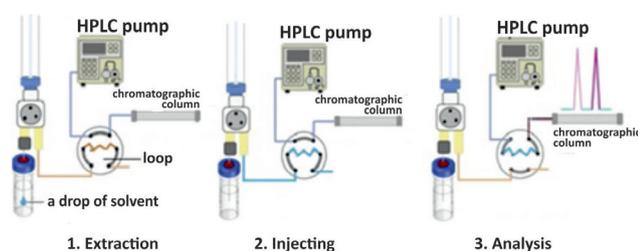
**Figure 3** A scheme of an automated SDME-LC procedure [9]
